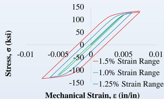
Figure 4: Three strain ranges for cube single element at 70°F
