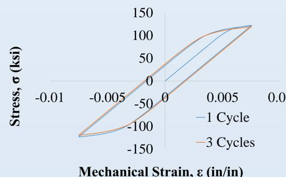
Figure 6: Comparison of one and three fully reversed cycle at 1.5% strain range and 70°F
