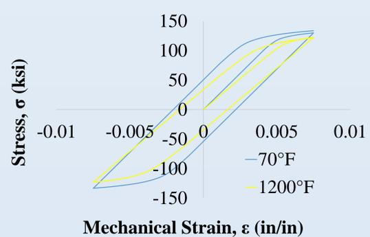
Figure 7: Comparison of hysteresis for 70°F and 1200°F with 1.5% Strain Range
