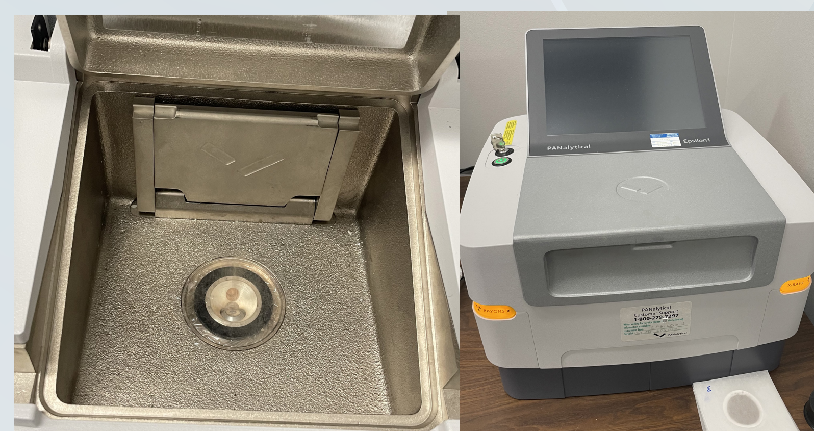
Figure 7: X-Ray Floresces Instrument
