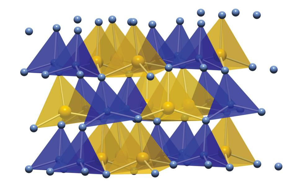
MgSiN<sub>2</sub> has many attractive properties such as high thermal conductivity, low dielectric constant, high hardness, high thermal stability, good oxidation resistance (up to 920°C) and high electrical resistance at room temperature
