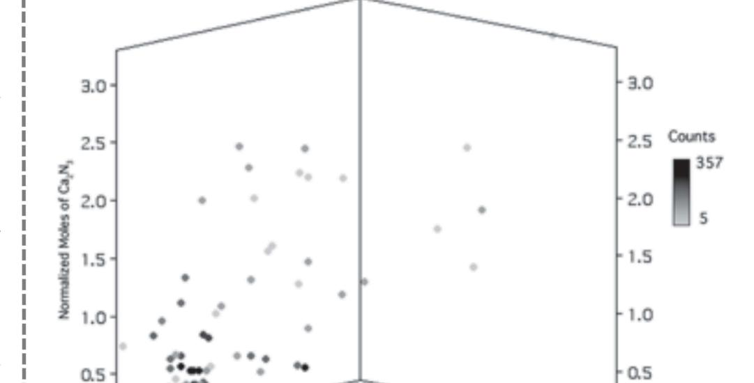
A map of reactions performed in a genetic algorithm search of the system:  $xSiO_2 + yMg_2N_3 + zLi_3N + wCa_3N_2$  MgSiN<sub>2</sub> + byproducts. The intensity of the most intense MgSiN<sub>2</sub> peak, in counts, is indicated by the color of each point. The intensity of MgSiN<sub>2</sub> peak is indicative of product crystallinity. The MgSiN<sub>2</sub> crystallinity was increased from 170 to 357 counts.
