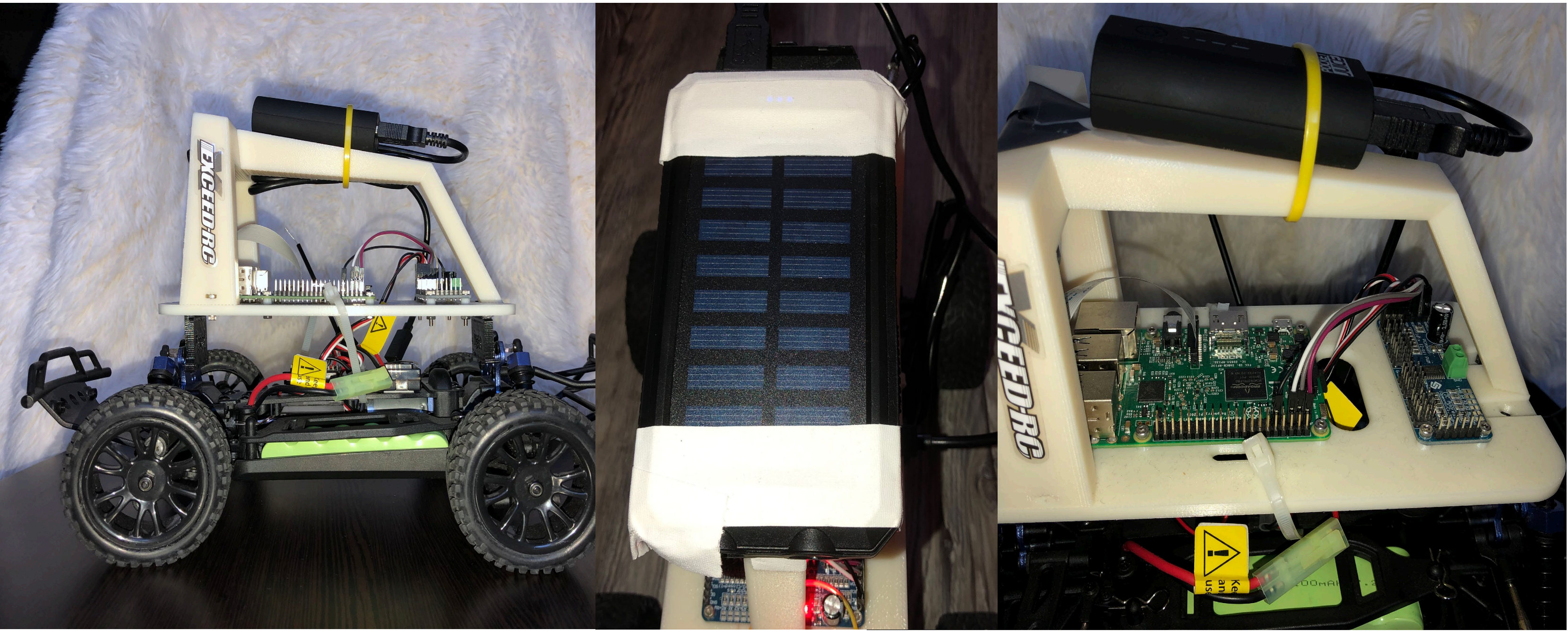
Figure 1: RC vehicle equipped with Raspberry Pi and solar panel
